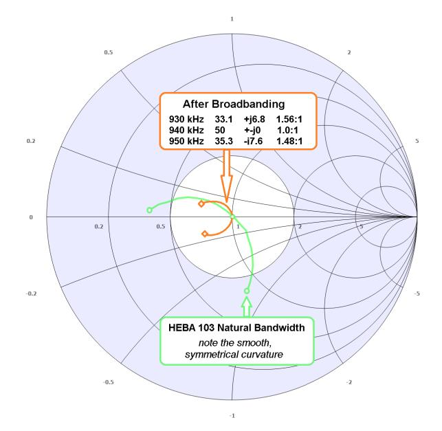
The Smith Chart above shows the actual measured bandwidth of the HEBA 103, within the 20 kHz channel of WGFP, in green. Kurt Gorman of Phasetek, **WWAS** Chief Engineer, recently redesigned the WGFP Antenna Tuning Unit with bandwidth-flattening design technology, so that All-Digital AM transmission performance will be quite good, as shown in orange.
